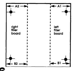
• Add 3.2 mm (1/8") to both open area measurements. Use utility knife to cut filler boards to fit.
